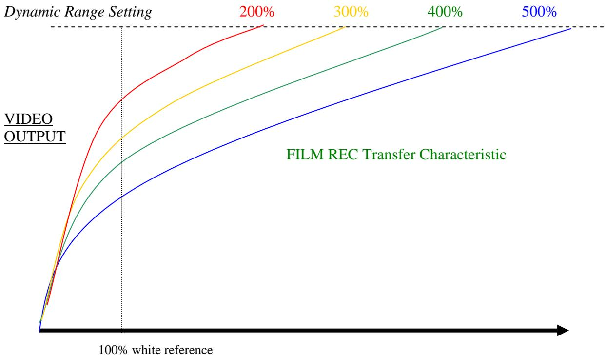
Reducing Dynamic Level increases the image contrast similarly to increasing the master gamma. If the full 500% is not needed for the scene content, more tonal levels can be used by the image if the dynamic level is decreased. This will also yield a more saturated image.
