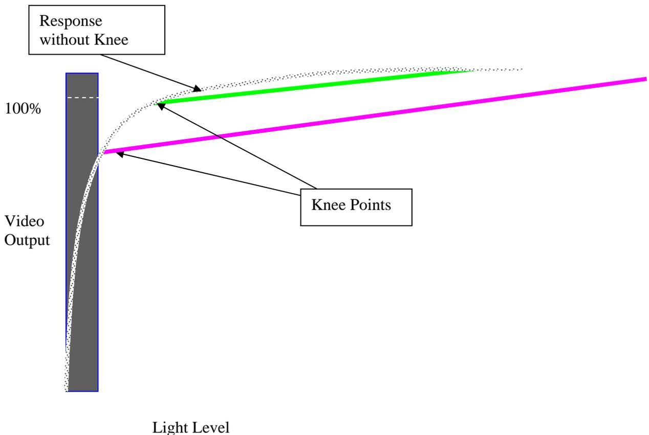
Aggressive knee adjustments attempt to mimic the film "shoulder" (the highlight portion of the film's negative's transfer characteristic). By lowering knee point and tweaking the knee slope the effective dynamic range can be increased.
